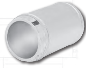
1G 1" Insulation 6" Diameter - 2" 8" - 18" Diameter - 3" 20" - 32" Diameter - 4" 34" - 42" Diameter - 5" 44" - 48" Diameter - 6"
